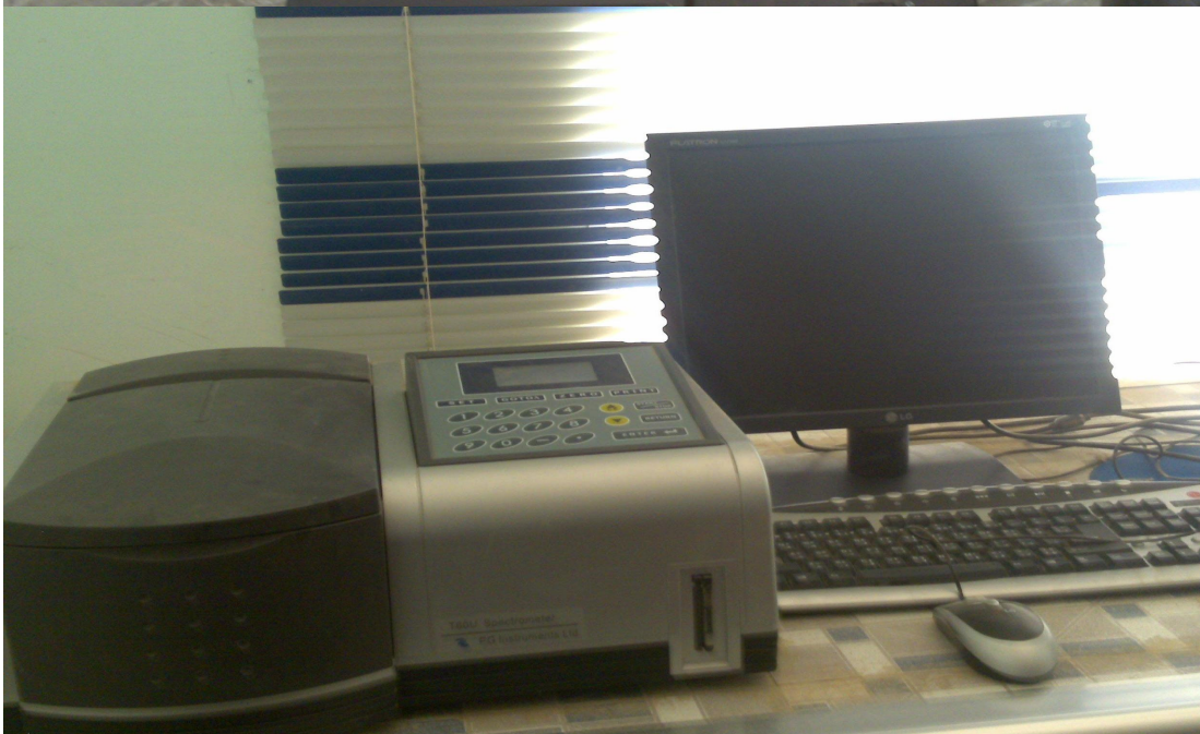
Figure (3) flame photometer that used in sodium content .measuring
